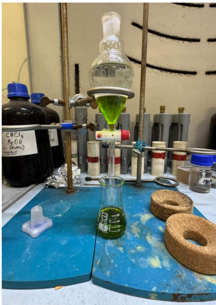
Figure 11. Liquid-liquid lipid extraction workflow included from the draft report.
