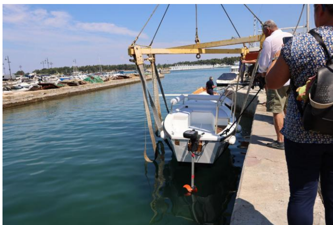
Modern batana afloat after crane handling; electric outboard visible.
