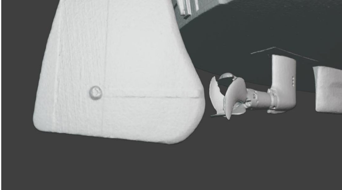
Rear underside view of the 3D model, showing the rudder blade and engine turbine clearly.
