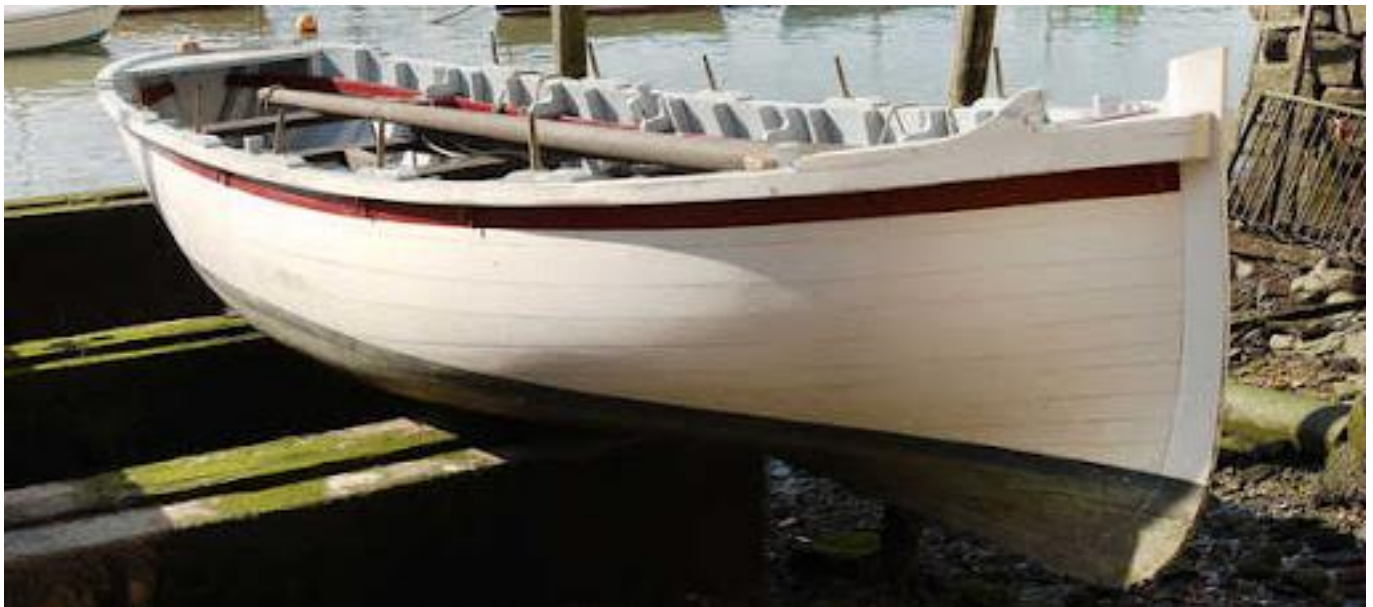
Figure 4 - Carvel-built vessel ( http://bertan.gipuzkoakultura.net/23/ing/11.php ).
