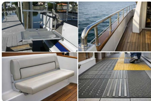
Figure 1. Key accessibility features on board: side-boarding ramp, external handrails, ergonomic lateral bench, and tactile flooring.
