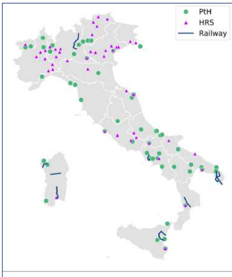
Figure 44 Future locations in Italy for hydrogen production plants (green dots), planned hydrogen refuelling stations for road transport (purple triangles), and railway lines to be converted to hydrogen (blue lines) Source: Gandiglio, M. et Marocco, P. (2024.)
