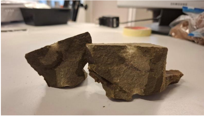
Figure 32 - Sandstone sample after testing: different water penetration patterns.
