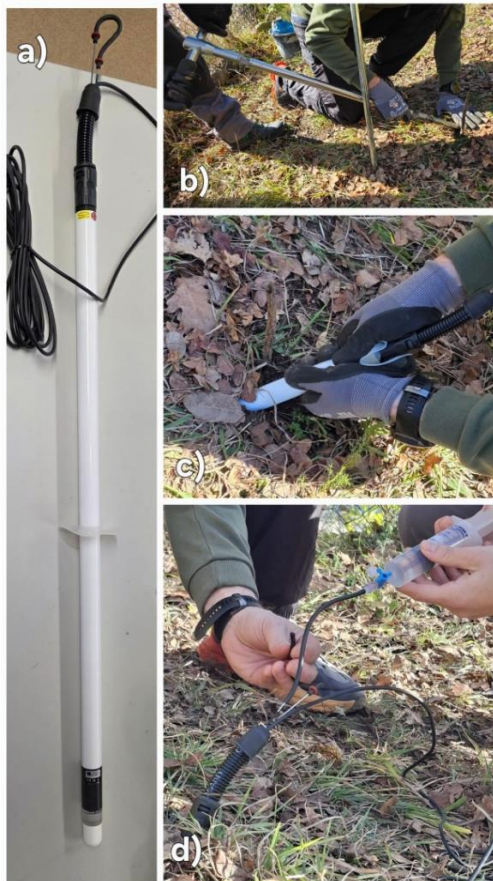
Figure 39 - a) TEROS 32; b) Drilling the hole with auger; c) Pushing TEROS 32 into drilled hole; d) Filling TEROS 32 with water syringe.
