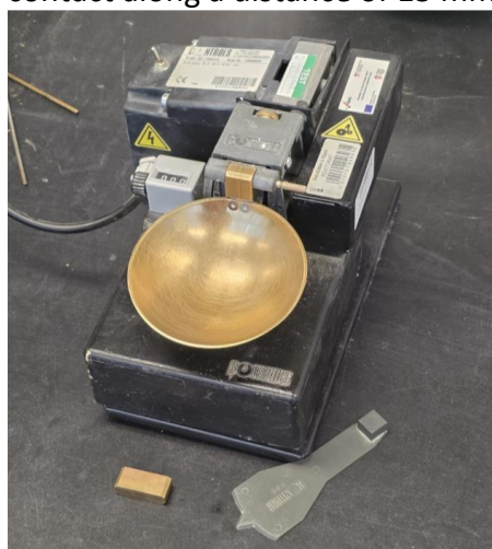
Figure 44 - The liquid limit device.
