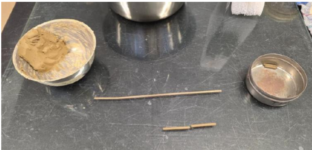
Figure 48 - Rolling of soil mass thread for plastic limit determination.
