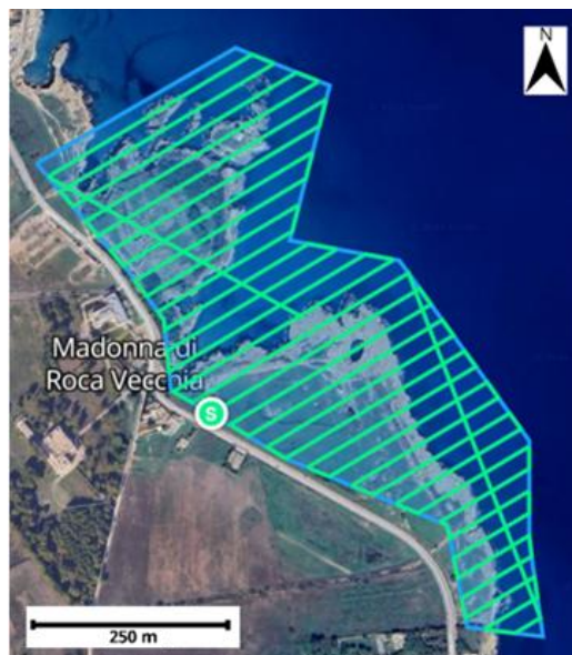
Figure 20 - DJI Mavic 3E vertical flight plan for the study area.
