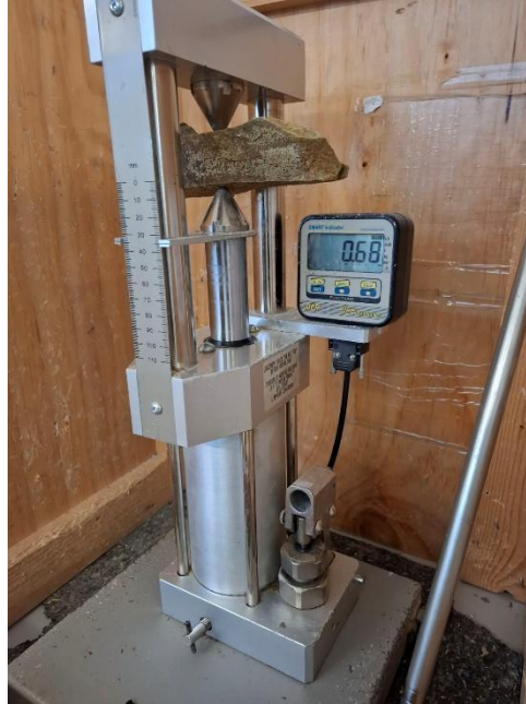
Figure 31 - Point Load test testing at the Geotechnical Laboratory, University of Rijeka, Faculty of Civil Engineering.
