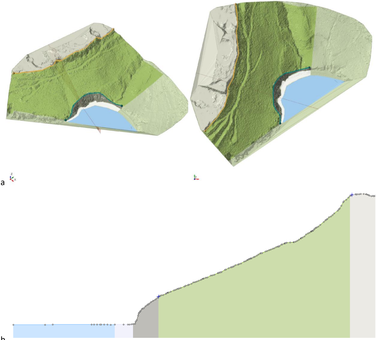
Figure 81 - a) 3D model with position of cross section in RocFall3 software, b) cross-section of the model in RocFall2 software showing regions with different material properties and the positions of seeder points.
