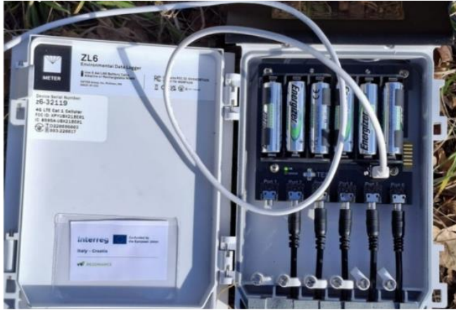
Figure 40 - Data on soil moisture content changes, as seen on ZENTRA Cloud service (top); and data logger ZL6 with all the instruments connected (bottom).
