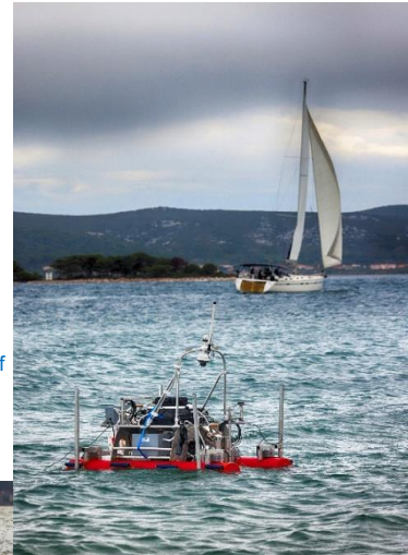
SWAMP-2 vehicle designed and developed to sample water and collect data in the stretch of water in front of tidewater glaciers in the Arctic (Hornsund, Spitsbergen)!
