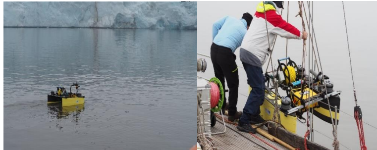
SWAMP-2 vehicle designed and developed to sample water and collect data in the stretch of water in front of tidewater glaciers in the Arctic (Hornsund, Spitsbergen)!
