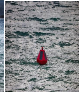
Smart Buoy - Innovative smart marine buoys contain a static buoy that collects, analyzes and stores measurements of various environmental values using built-in sensors
