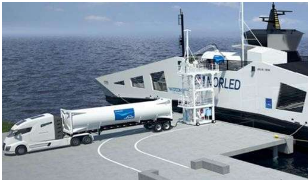
Figure 5 LH2 bunkering facility for ships, custom-designed for the MF HYDRA
