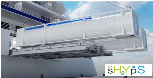
Figure 10-3 Liquid hydrogen tanks based on swappable concept developed in sHYpS EU co-funded project
