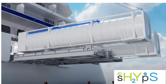
Figure 8-4 Liquid hydrogen tanks based on swappable concept developed in sHYpS EU co-funded project
