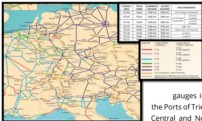
Figure 22 European railway network: loading gauge of the main lines
