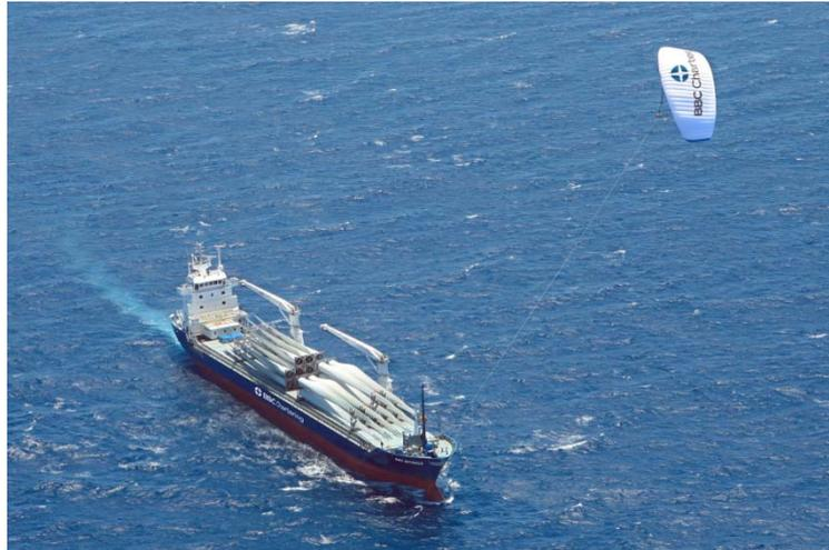
Figure 1. Towing kite system, [20]
