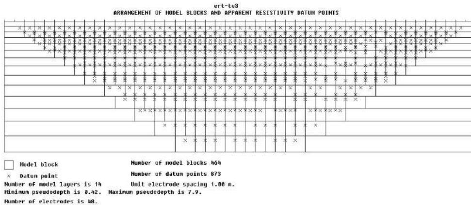
**Fig. 5.** Initial model in the resistivity inversion program RES2DINV.
