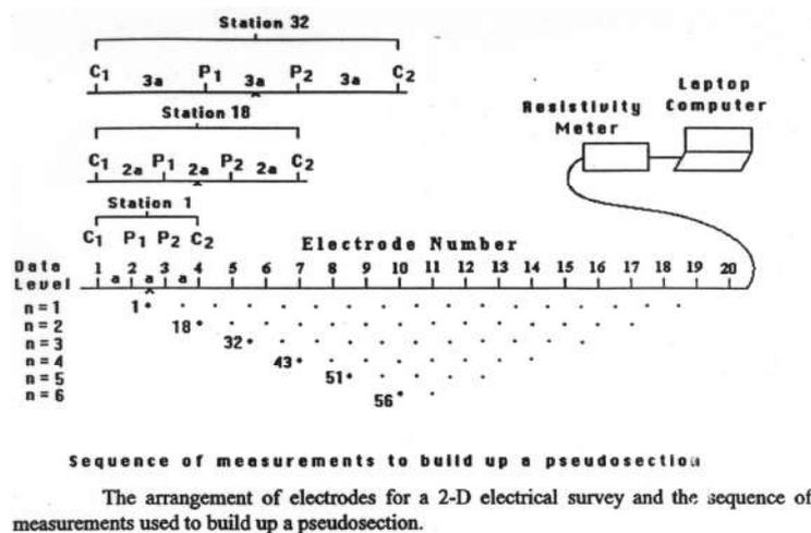
**Fig. 4.** Electrical quadripoles along a 2-D survey. Cx:current electrodes; Px: potential electrodes.
