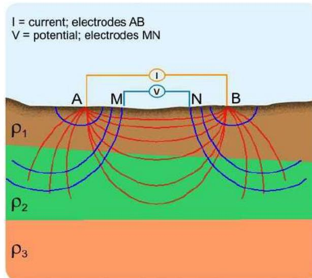
**Fig. 3.** Electrical quadrupole A and B: current electrodes; M and N: potential electrodes.
