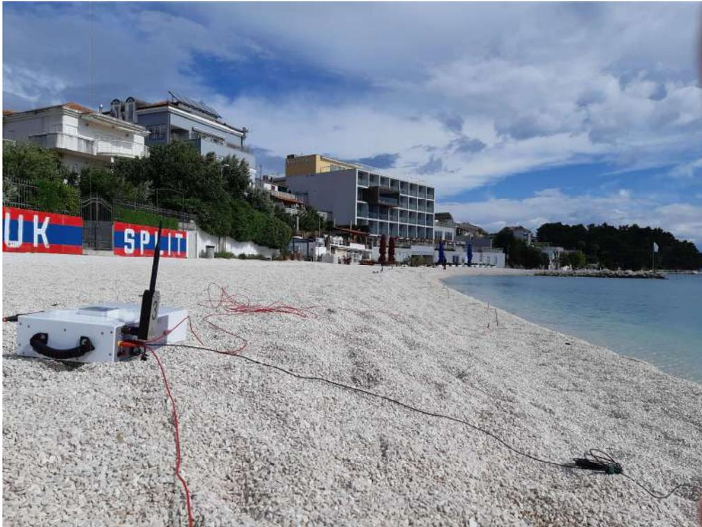
**Fig. 9.** Field operations with the MultiSource Wireless Acquisition System in the Podstrana beach
