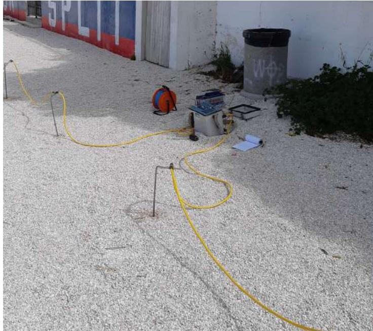
**Fig. 6.** Particular of the electrode coupling in the Podstrana beach
