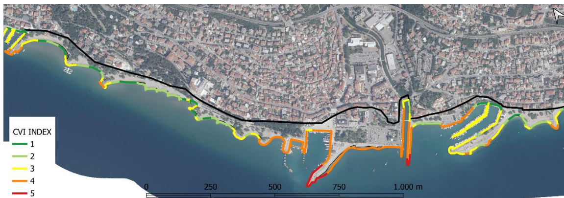
Figure 1. Coastal vulnerability of the Crikvenica shoreline (section between Crni mol and Podvorska), based on the Coastal Vulnerability Index methodology of Ružić et al. (2022).
