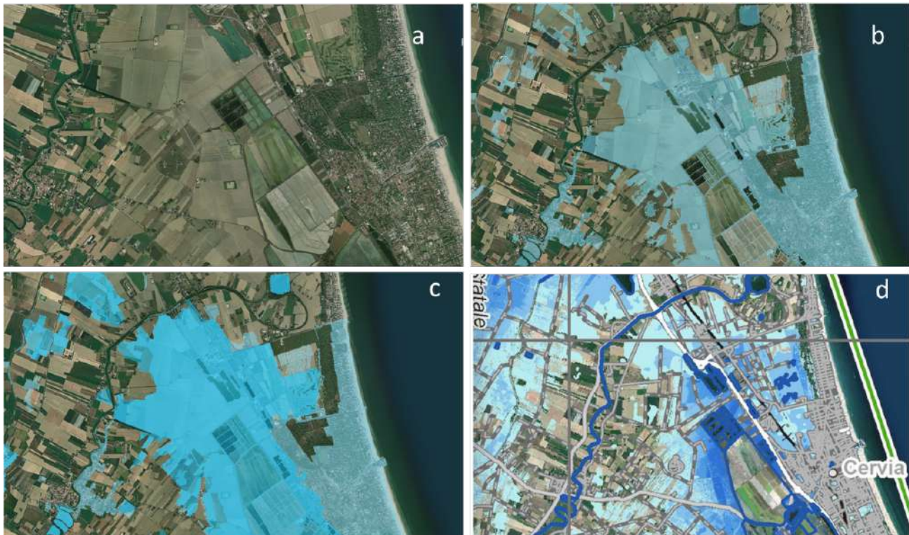
Figure 4: The 2023 flood in the Cervia saltworks a) the saltworks before May 16; b and c) flood propagation dynamics May 16 and 17; d) maximum flood depth between May 16 and 23: water depth (m) ranges from light blue (0–0.5) to dark blue (3.5–5.5).
